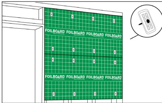
**STEP 4** Fasten the Foilboard panel to the stud-work with Foilboard fasteners. Use 4-6 fasteners per square metre.
