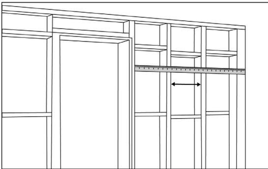
**STEP 1** Measure the required area, then mark the Foilboard panel before cutting to size.
