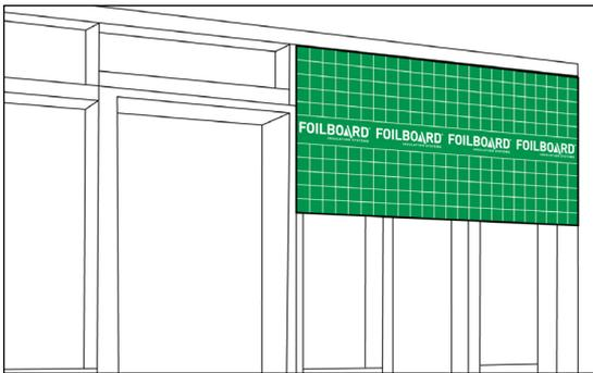
**STEP 3** Position the Foilboard panel against the outside the stud-work with the anti-glare side facing out. Take care not to leave any gaps.
