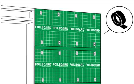
**STEP 5** Tape any joins or gaps using Foilboard green joining tape.
