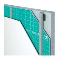
Incorporating Foilboard® GREEN rigid insulation panel into a standard 150mm concrete precast system, you can dramatically increase the thermal performance of the wall from an R0.3, to R2.8,
