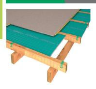
Through the utilisation of the Foilboard® Floor Saddles, Foilboard® GREEN rigid panel can be installed quickly and easily into the sub-floor before laying timber / particle board flooring.
